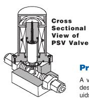
PSV Proportionating Electromagnetic Valves are designed to respond to variable power inputs to regulate the flow of liquids and gases proportionately.
