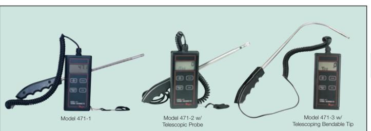
The Series 471 Digital Thermo Anemometers are versatile dual function instruments that quickly and easily measure air velocity in four field selectable ranges, in either feet per minute or meters per second, plus air temperature in °F or °C. High contrast LCD display shows both range selected and present velocity. Convenient backlight provides perfect visibility in low light conditions. Light automatically shuts off after 2-1/2 minutes to prolong battery life. Low battery warning is included.
