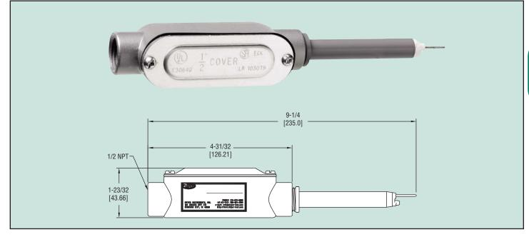
**The Series 641B Air Velocity Transmitter** uses a heated mass flow sensor technology. It has 4 user-selectable ranges from 250 FPM to 2000 FPM with corresponding metric ranges of 1.25 MPS to 10 MPS. The 641B provides an isolated 4-20 mA output proportional to the velocity.
