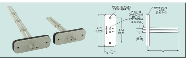
**The Series PAFS-1000 Averaging Flow Sensor** is ideal for sensing differential pressure in the inlet section of variable air volume terminal units and fan terminal units. Units can also be used to sense differential pressure at other locations in the main or branch duct systems.
