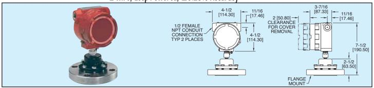
Series PLT Piezoresistive Level Transmitters provide reliable measurement and control of process levels by sensing the hydrostatic pressure in a tank. The loop-powered level transmitter delivers a 4 to 20 mA output signal proportional to hydrostatic pressure and specific gravity of the fluid for indicating, recording or control purposes. Easily accessible zero and span potentiometers make calibration in the field quick and simple. Units are equipped with EMI and reverse polarity protection.
