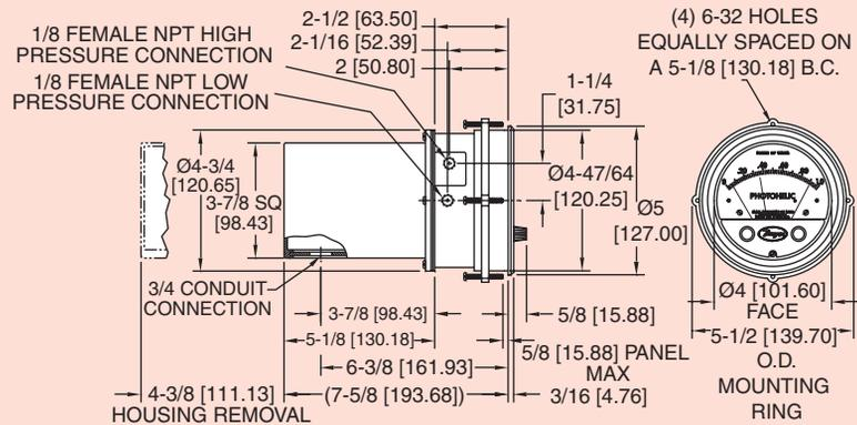
**Photohelic® Switch/Gages** function as versatile, highly repeatable pressure switches combined with a precise pressure gage employing the time-proven Magnehelic® design. The Photohelic® measures and controls positive, negative or differential pressures of air and compatible gases. Standard models are rated to 25 psig (1.7 bar) with options to 35 (2.4) or 80 (5.5 bar) psig. Single pressure 36000S models measure to 6000 psig (413 bar) with a 9000 psig (620 bar) rating.
