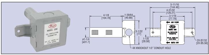
The Model CDD Duct Mount Carbon Dioxide Transmitter monitors the occupancy in a room by detecting the concentration of carbon dioxide in the return air duct. The non-dispersive infrared sensing technology automatically updates the calibration of the transmitter using a proprietary logic feature which limits the amount of error due to drift. The Model CDD can measure up to 2000 PPM in duct air flows less than 1500 FPM.
