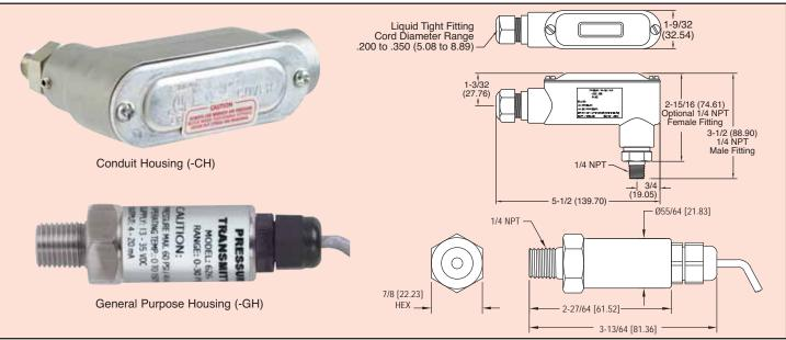
The Series 626 Pressure Transmitters possess a highly precise 0.25% piezo-resistive sensor contained in a compact, rugged, NEMA 4X stainless steel general purpose housing or cast aluminum conduit housing.
