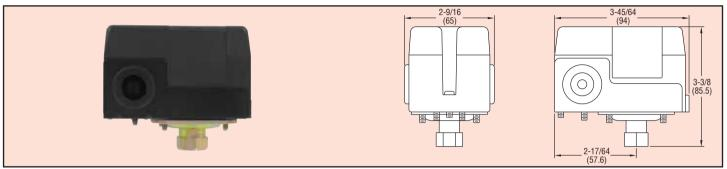
The Series CXA Water Pump Pressure Switches have been proven reliable for controlling automatic water systems. These switches are very popular for use on water pumping systems. The set point and deadband are both easily adjustable via screws inside the cover. For ease of installation, the switches come with a 1/4" female NPT process connection and can be mounted in any orientation. The series CXA's simple design makes it a great switch for an installer at any skill level.
