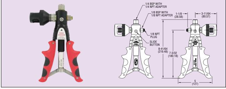
The Series PCHP Pneumatic Hand Pump comfortably sources pressure and vacuum to check calibration of gages, switches, transmitters, and recorders. The contoured cushion handles provide extra comfort while preventing the pump from sliding. The oversized check valve provides smooth operation throughout the output range. The dual o-rings on all pistons ensure zero leakage.
