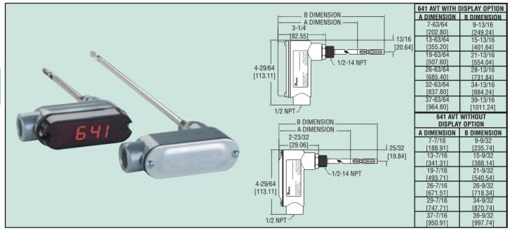
The new Dwyer Series 641 Air Velocity Transmitter is the ideal instrument for monitoring air flow. This transmitter uses a heated mass flow sensor which allows for precise velocity measurements at various flow rates and temperatures. The 641's 16 field selectable ranges provides it the versatility to be selected for several air flow applications. The optional LED produces a complete, low-cost solution for local indication of air flow.
