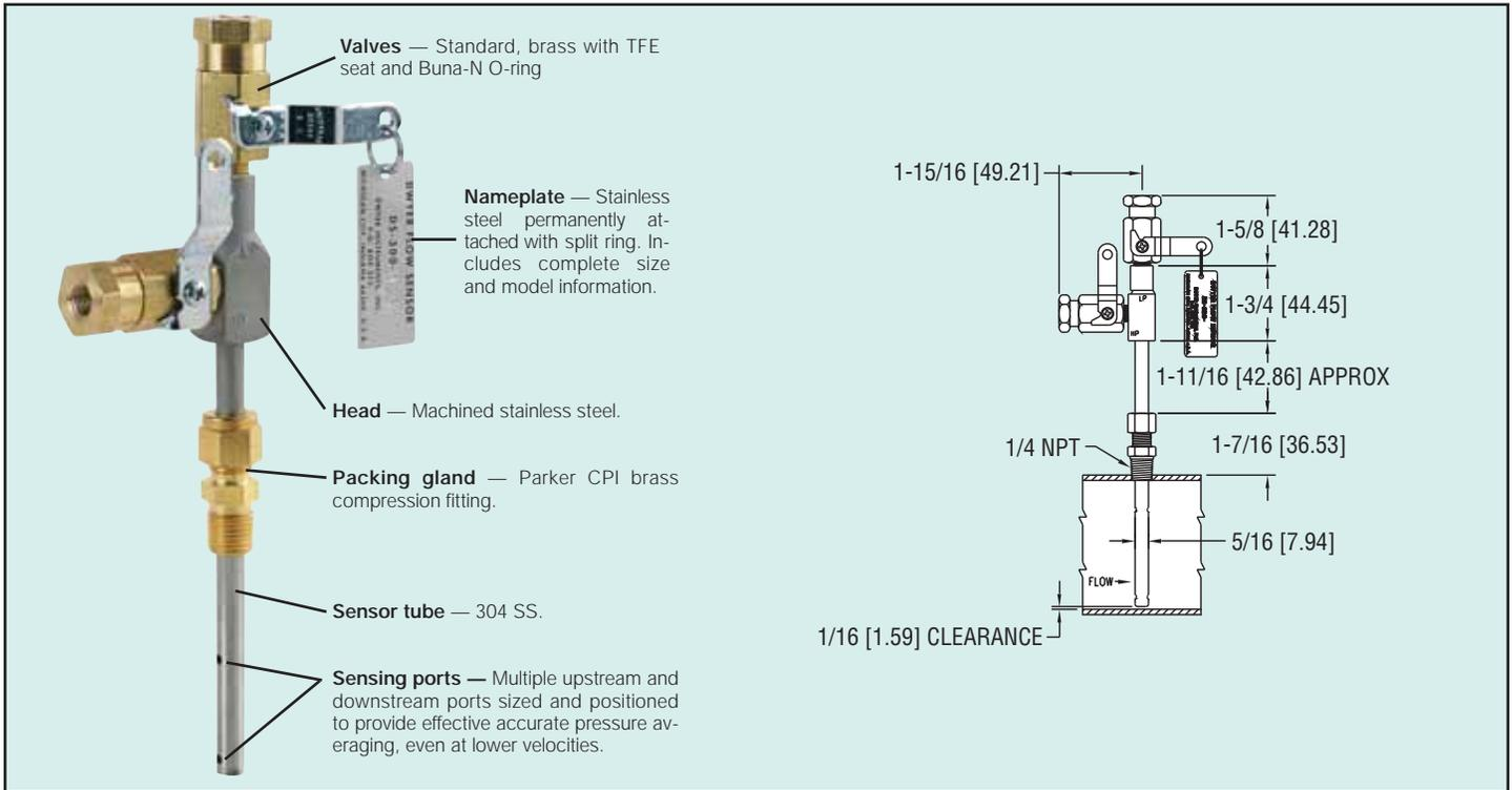
**In-Line Flow Sensors** are averaging Pitot tubes that provide accurate and convenient flow rate sensing for schedule 40 pipe. When purchased with a Dwyer® Capsuhelic® differential pressure gage of appropriate range, the result is a flow indicating system delivered off the shelf at an economical price.
