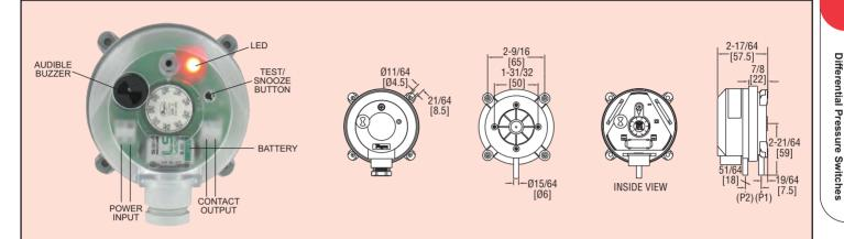
**The Series BDPA Adjustable Differential Pressure Alarm** with built-in audible and visual set point indication is designed for overpressure, vacuum, and differential pressure applications. The scaled adjustment knob allows changes to the switching pressure to be made without a pressure gage. The BDPA is available with settings from 0.08 in w.c. (20 Pa) to 20 in w.c. (5000 Pa). The silicone diaphragm and PA 6.6 body make the Series BDPA perfect for use with air and other noncombustible gases.
