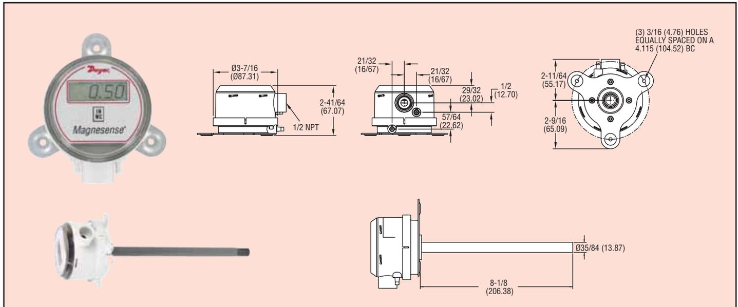
The Series MS Magnesense® Differential Pressure Transmitter is an extremely versatile transmitter for monitoring pressure and air velocity. This compact package is loaded with features such as:
