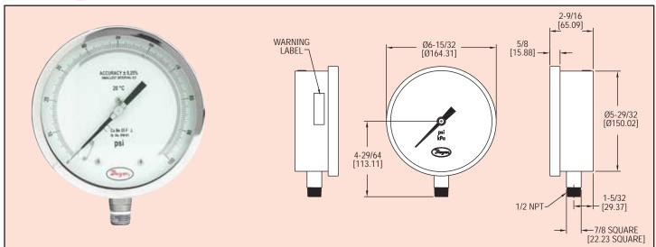
The Series SGR/SGJ Gages have dual English/metric scales with  $\pm 0.25\%$  ASME Grade 3A accuracy, and contain a green dial with antiparallax mirror for ease of reading measurements by the user.
