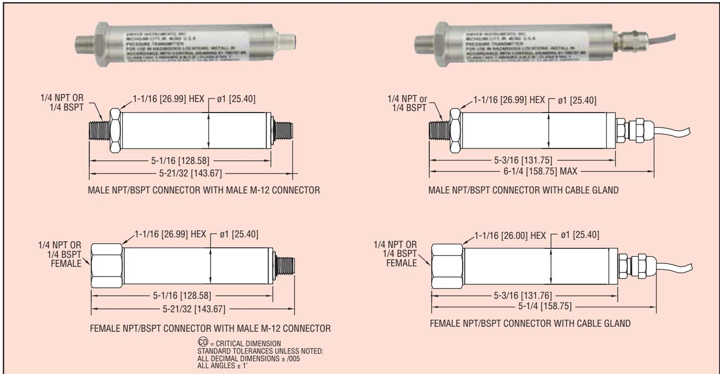
The Series IS626 Intrinsically Safe Pressure Transmitters convert pressure into a standard 4-20 mA output signal. The Series IS626 can be used to accurately measure compatible gases and liquids compatible with its 316/316L Stainless Steel wetted parts. Series IS626 full scale accuracy is 0.25%. Designed for industrial environments with a NEMA 4X (IP66) housing, this transmitter resists most effects of shock and vibration. Models are available with a 3' cable or M-12 4 pin connection.
